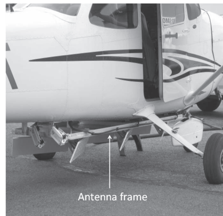
Fig. 1. Antenna frame (arrow) installed on a Cessna 172. Both antennas radiate toward the starboard side of the aircraft.
