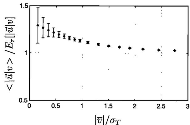
**Figure 9.** The means (diamonds) and standard deviations (vertical bars) of the ratio  $\langle |\vec{u}|v \rangle / E_r[|\vec{u}|v]$  versus  $|\bar{v}|/\sigma_T$ . The observed  $\langle |\vec{u}|v \rangle$  is used, and  $E_r[|\vec{u}|v]$  is based on the observed  $\bar{u}$ ,  $\bar{v}$ , and  $\rho_{uv}$ , but with 80% of the observed  $\sigma_u$  and  $\sigma_v$ . The corresponding result using the observed  $\sigma_u$  and  $\sigma_v$  is shown in Figure 7a.
