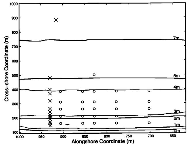
**Figure 1.** Locations of the 13 Duck94 (crosses) and 26 SandyDuck (circles) current meters used in this study. The U.S. Army Corps of Engineers Field Research Facility (FRF) coordinate system is used. Bathymetry from October 2, 1997, is contoured in units of meters below mean sea level.
