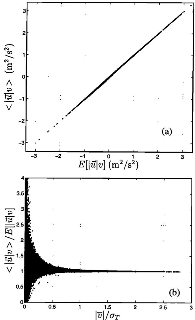
**Figure 4.** (a) Observed  $\langle |\bar{u}|v \rangle$  versus the expected value  $E[|\bar{u}|v]$  assuming a joint-Gaussian velocity field with observed means, variances, and  $\rho_{uv}$ . The slope is 1.00, and the skill is  $r^2 = 1.00$ . (b) The ratio  $\langle |\bar{u}|v \rangle / E[|\bar{u}|v]$  versus  $|\bar{v}| / \sigma_T$ .
