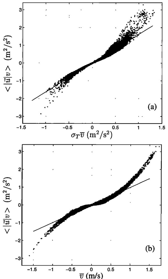
**Figure 2.** (a) Observed  $\langle |\bar{u}|v \rangle$  versus  $\sigma_T \bar{v}$ . The solid line is the least squares best fit (slope  $a = 1.62$  and skill  $r^2 = 0.94$ ). (b) Observed  $\langle |\bar{u}|v \rangle$  versus  $\bar{v}$ . The solid line is the least squares best fit (slope = 0.99 m/s and skill  $r^2 = 0.88$ ). Each panel has 70,099 data points.
