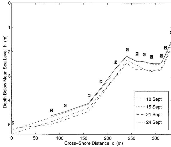
FIG. 6. Depth profiles and sensor locations (squares) of the four field data case studies.
