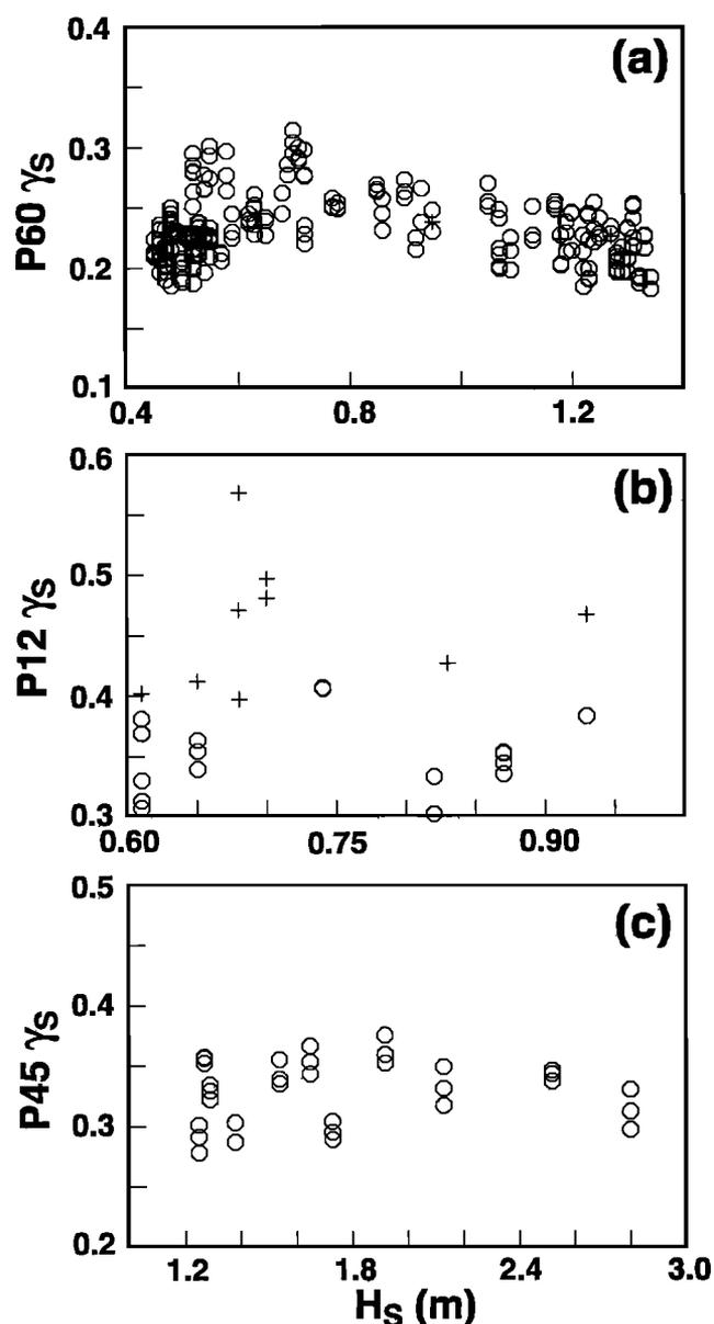
Figure 2. Ratio ( $\gamma_s$ ) of significant sea swell wave height to water depth versus deep water significant wave height,  $H_s$ , for depths greater than (circles) and less than (pluses) 0.8 m at (a) P60 at San Onofre, (b) P12 at Scripps, and (c) P45 at Duck.
