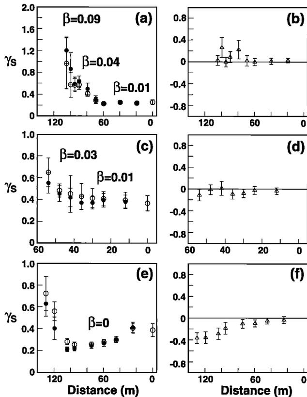
**Figure 6.** Observed (open circles) and predicted (solid circles) average and standard deviation (vertical bars) of  $\gamma_s$  at each sensor for all runs at San Onofre (Figure 6a), Scripps (Figure 6c), and Duck (Figure 6e). The average (triangles) and standard deviation of normalized prediction errors  $\{[(\gamma_s)_{\text{pred}} - (\gamma_s)_{\text{obs}}]/(\gamma_s)_{\text{obs}}\}$  are shown for all runs at San Onofre (Figure 6b), Scripps (Figure 6d), and Duck (Figure 6f).
