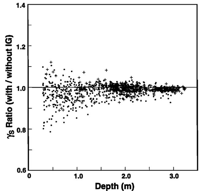
Figure 10. Ratio of  $\gamma_s$  predicted by the numerical model initialized with the total ( $0.004 \leq f \leq 0.18$  Hz) sea surface and velocity fluctuation time series to  $\gamma_s$  predicted by the model initialized with band-passed ( $0.05 < f \leq 0.18$  Hz) time series versus water depth for San Onofre (solid circles,  $0.45 \leq H_s \leq 1.34$  m) and Duck (pluses,  $1.2 \leq H_s \leq 2.8$  m) data.
