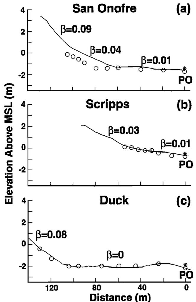
**Figure 1.** Locations of pressure sensors (circles) and current meters (asterisks), and approximate beach slopes,  $\beta$ , at (a) San Onofre, (b) Scripps, and (c) Duck. The  $x$  axis, positive onshore, is zero at the sensor location where the numerical model is initialized.
