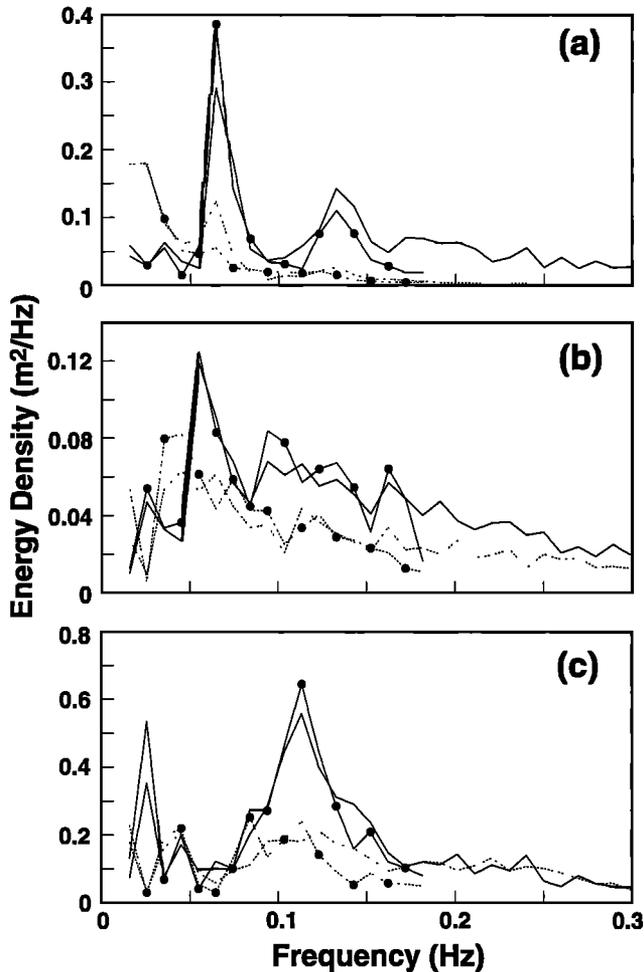
Figure 4. Observed (lines) and predicted (lines with solid circles) sea surface elevation energy density spectra at sensors (a) P60 (solid lines) and P95 (dotted lines) at San Onofre, (b) P12 (solid lines) and P36 (dotted lines) at Scripps, and (c) P45 (solid lines) and P105 (dotted lines) at Duck.
