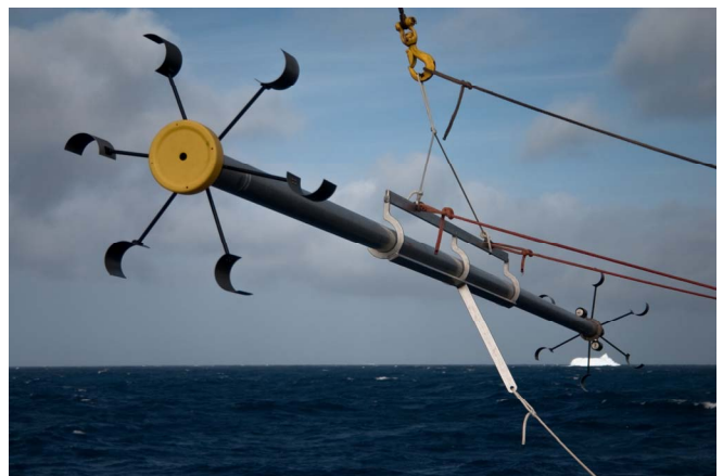
Figure 1. A DIMES Shearmeter is shown. The plastic cover on the lower (near) end of the float protects the oil bladder for the buoyancy pump. The shear-sensing vanes are shown. Photo by Uriel Zajackovski.
