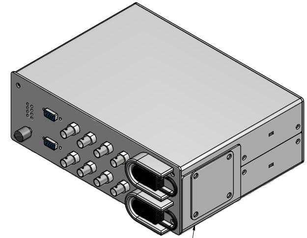
Rack Mount Ears Shown in Stowed Position
