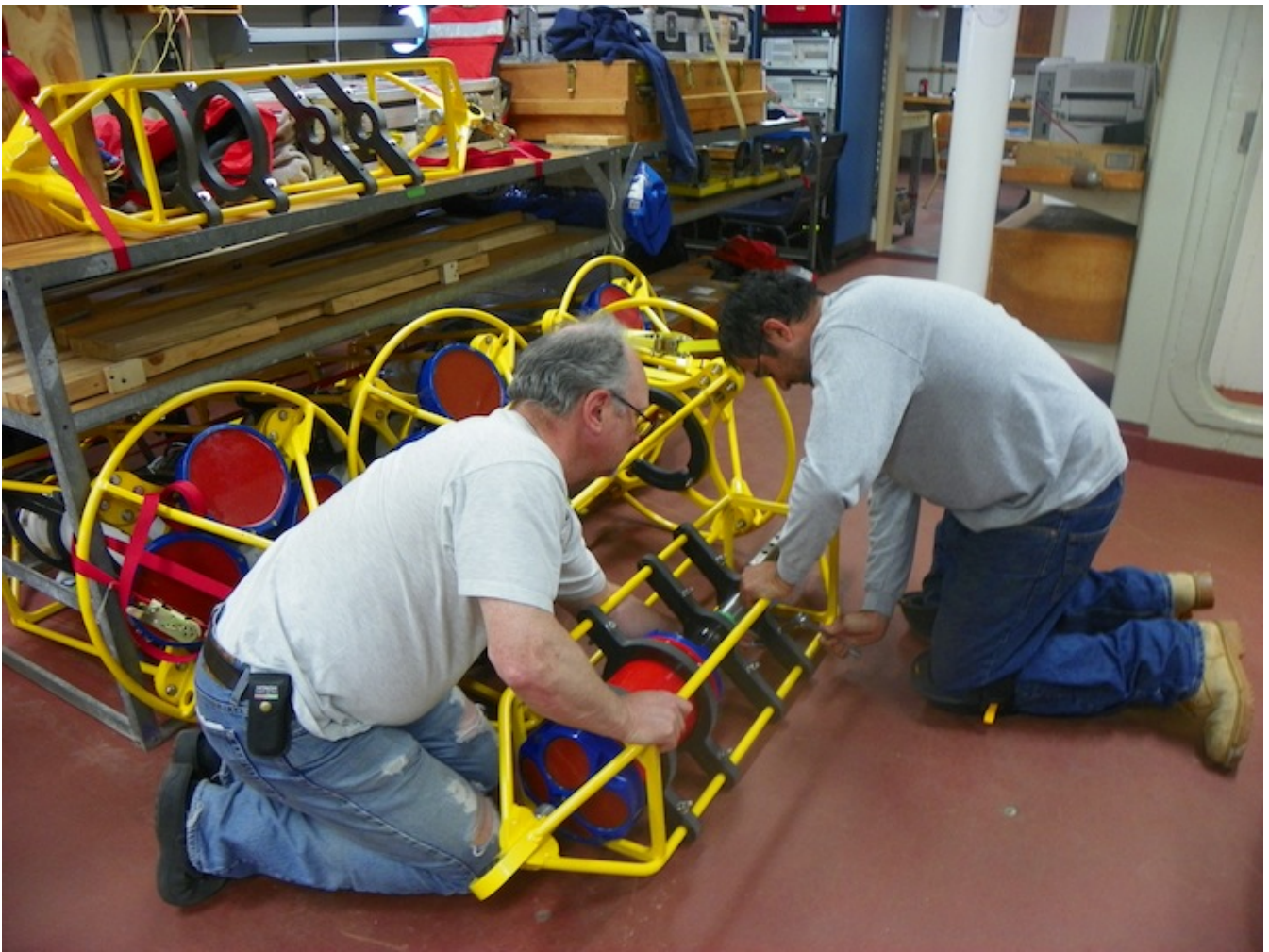
Magnus Danielsen and Dan Torres ready an ADCP to be placed on a mooring in the Denmark Strait to collect data for a year. © Pat Keoughan
