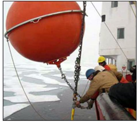
Top flotation sphere being attached at the end of the deployment.
