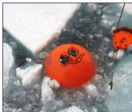
Spherical top float being recovered in the ice.
