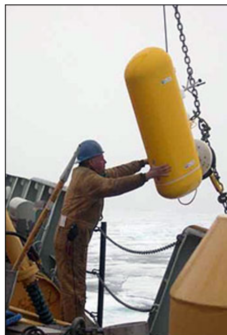
John Kemp recovering the McLane Moored Profiler.
