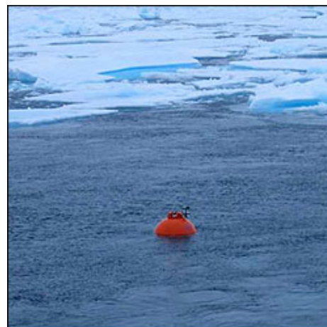
The WHOI-A top flotation package reaching the surface after being deployed beneath the ice for one year.
