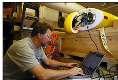
Rick Krishfield programs the CABOS moored profiler for tomorrow's deployment.
