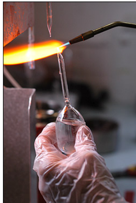
Nes Sutherland seals glass bottles of water samples with a propane torch.
