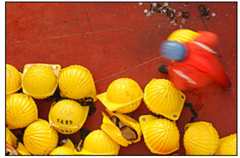
Recovered floats. Notice the crushed float in the center.
