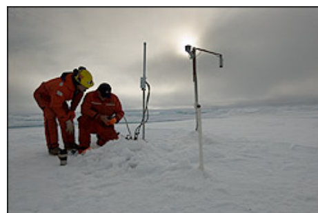
Doug Sieberg (left) and Rick Krishfield (right) give the Ice Mass Balance buoy a final checkover.
