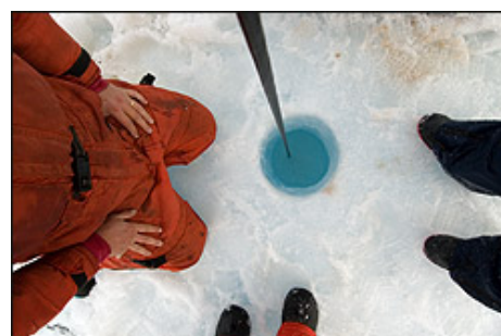
An expectant mooring team watches 800 meters of line spool off into the depths. The profiler will make four trips a day up and down this wire collecting
