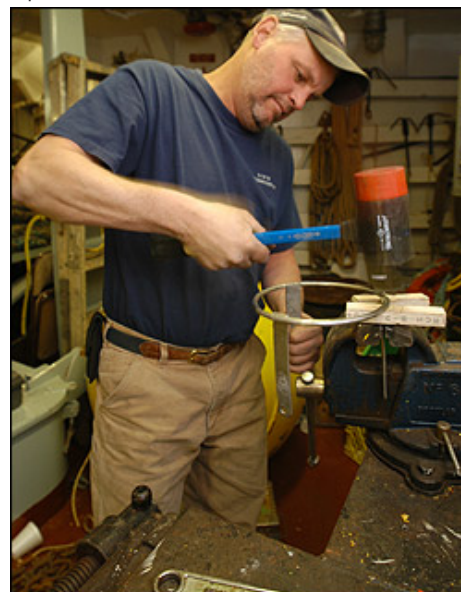
Body and fender work... John Kemp repairs the cage protecting the upward-looking sonar on Mooring B's top sphere. The cage was crushed when the mooring popped up underneath an ice floe during the recovery.
