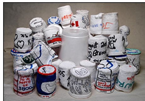
Oceanographic art--take styrofoam cup, add decoration, compress with 400 atmospheres of pressure. Cup in the middle is original size for scale.
