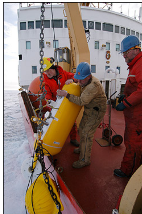
Doug Sieberg and John Kemp pull the moored profiler on deck (and a small tangle of floats).
