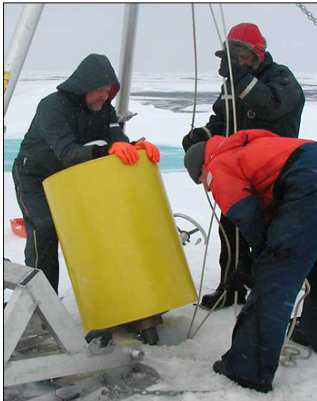
The ITP surface buoy is eased over the ice hole by Rick Krishfield while Will Ostrom and Kris Newhall gently lower the underwater mooring system using a tag line. Photo by Gary Morgan.
