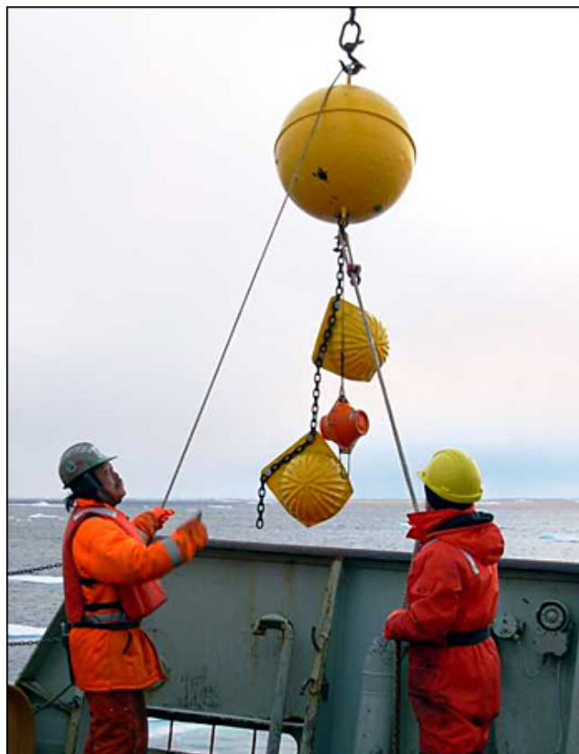
The top floatation of the CABOS mooring is brought on deck by Rico Amamio and Bill May. Photo by Rick Krishfield.
