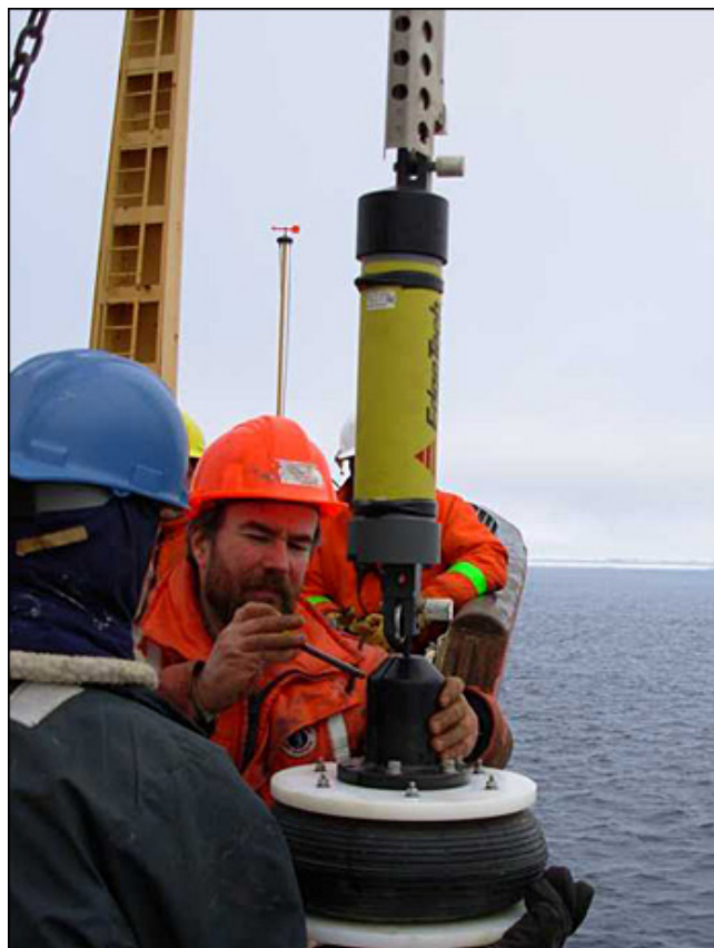
During the redeployment only hours later, Mike Dempsey attaches the profiler bumper to the mooring wire below the top transponder and temperature and salinity recorder. Photo by Rick Krishfield.
