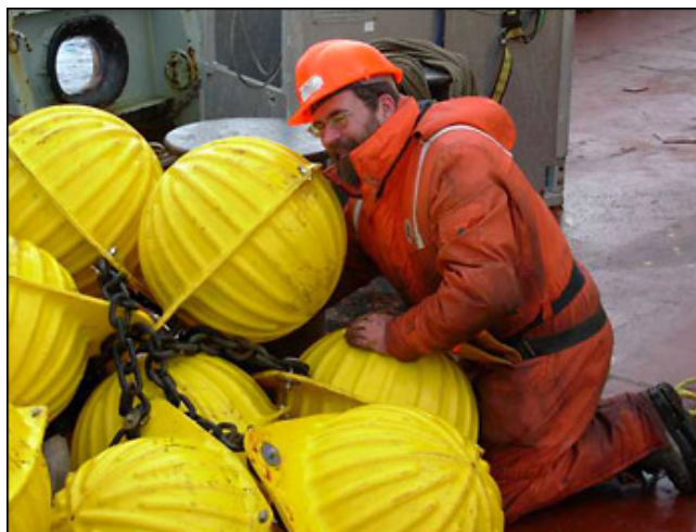
The author getting his hands wet (and dirty) for oceanography by decoupling flotation spheres during a mooring recovery. Photo by Rick Krishfield, WHOI.
