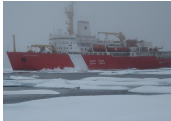
The ship is visible through the fog. The wake on the port bow is from the ship's bubbler system.
