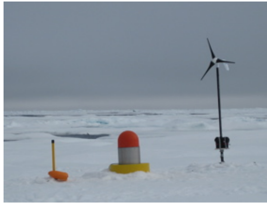
WHOI deployed this AOFB system to measure changes in ocean currents under the ice. It is powered by a battery that is recharged with wind energy.
