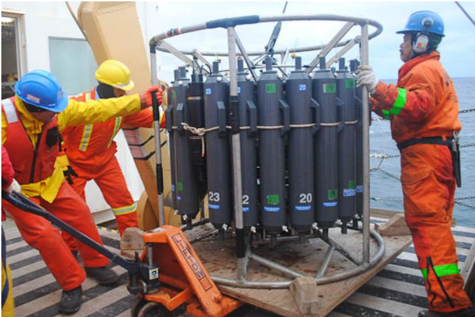
Crewmen Derrick Stone and Rico Amamio help Fisheries and Oceans Canada chemist Glenn Cooper haul in the rosette, a device used for obtaining water samples from specified depths. The data obtained in the rosette casts will be used for analysis and in papers, but the process of obtaining the data requires physical work.
