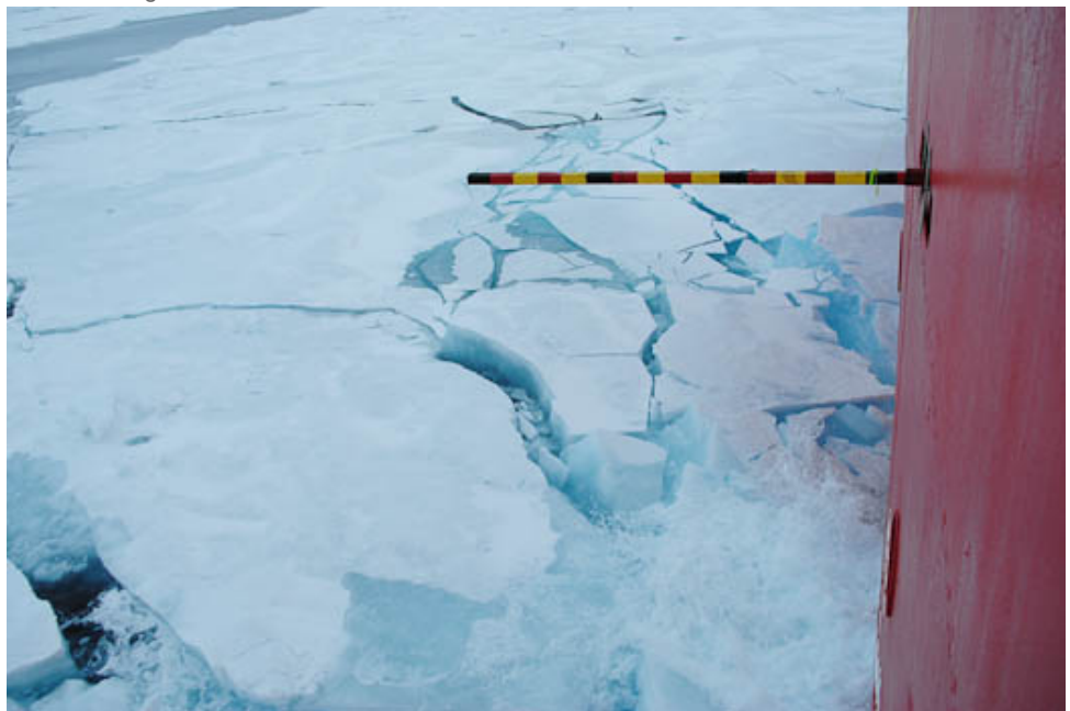
Ice breaking in progress. Notice how the ocean water splashes against the side of the ship. The red, yellow, and black stick in the foreground, jokingly called the "German flagpole," is used to estimate the thickness of fragments as they float by the side of the ship. Each block of color spans ten centimeters.
