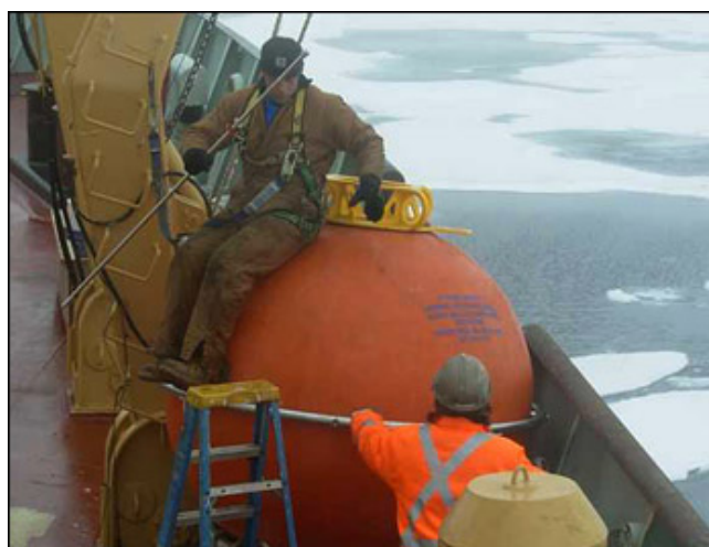
Kris Newhall prepares to install a tie rod on the sphere after installing a new top bracket which was dented when the top float surfaced under an ice floe during the recovery. Photo by Rick Krishfield, WHOI.
