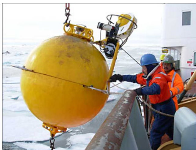
The ship's crane wire hooks to a lifting eye on the sphere.
