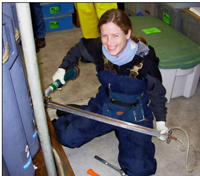
After the package is safely back in its container, Abby Spieler draws water from the rosette bottles into special copper tubes for Tritium and Helium analysis. Photo by Rick Krishfield, WHOI.
