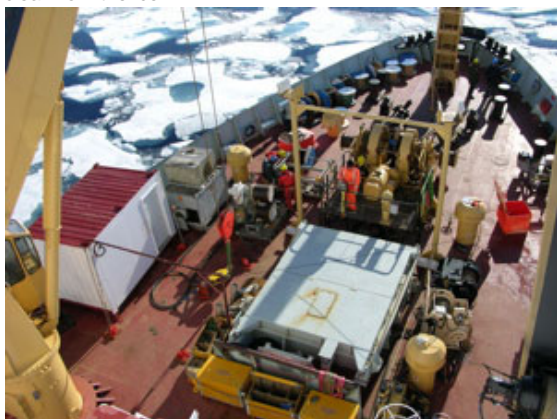
The mooring recoveries and deployments are staged from the foredeck. The Lebus winch can be seen on the port side (left), and the wire goes over the side through the A-frame on the starboard side (off the picture, to the right).
