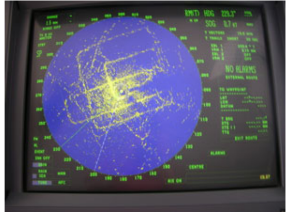
Radar are essential for navigation in the ice. Ridges are a strong targets, and areas of open water have little return intensity. This picture, however, was taken just before the recovery of mooring B, in fairly homogeneous first-year ice. Before releasing the float, we broke the ice around the mooring location in a square pattern. The rubble of broken ice along the ship's track is picked up here by the radar, in a 3-mile radius around the ship's location (in the center). Photos by Luc Rainville
