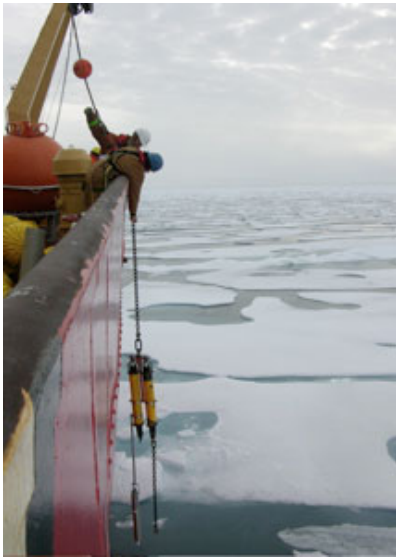
After a few hours, the acoustic releases, which held the whole mooring attached to the anchor for the past year are finally coming on board.
