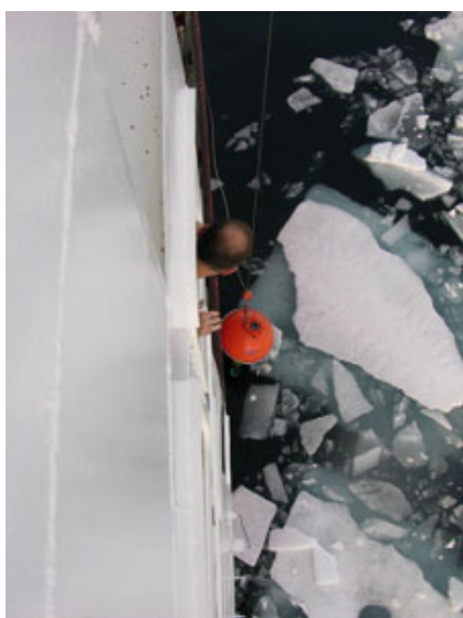
The sub-surface float (big orange ball) is on the surface! The Captain is looking out of the bridge to align it with the side of the ship.
