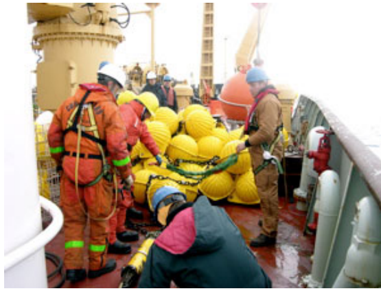
The whole mooring is on deck! The cluster of yellow balls is a bunch of glass spheres that add buoyancy to the mooring, here near the acoustic releases.
