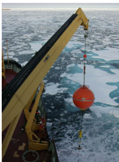
After hooking up the sphere, you have to lift it out of the water and connect the mooring wire to the winch.
