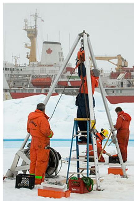
Placing an ice-tethered profiler in the pack ice.
