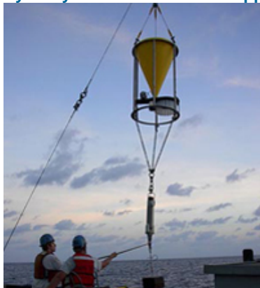
Deployment of a time-series sediment trap mooring for larval collections at the East Pacific Rise, 9°N (Stace Beaulieu)
