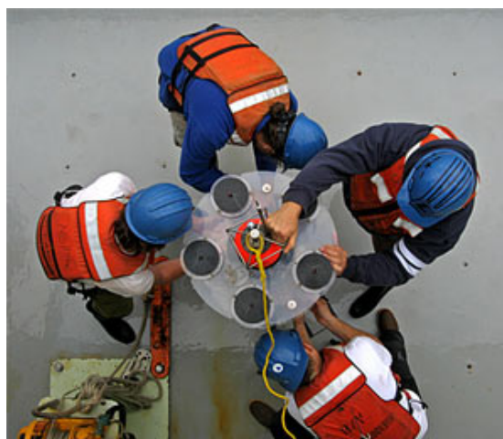
FIGURE 1: An array of sampling technologies were utilized in the VERTIGO program to follow the fate of particles sinking from sunlit surface waters through the ocean’s dimly lit twilight zone. In particular, Ken Buesseler and engineer Jim Valdes designed a new-generation neutrally buoyant untethered vehicle called the Twilight Zone Explorer, that is swept along with the currents and surfaces periodically to relay data via satellite. (Illustration by Jack Cook, Woods Hole Oceanographic Institution)
