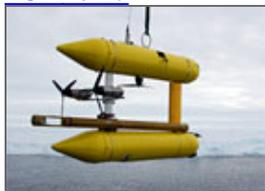
Also known as the "plume mapper," the Puma autonomous underwater vehicle uses sonar, lasers, and chemical sensors to search wide areas near the ocean floor and detect the telltale temperature, chemical, or particulate signals from hydrothermal vent plumes.
