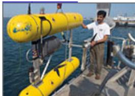
*SeaBED* is an AUV that can fly slowly or hover over the seafloor to depths of 6,000 feet (2,000 meters), making it particularly suited to collect highly detailed sonar and optical images of the seafloor.
