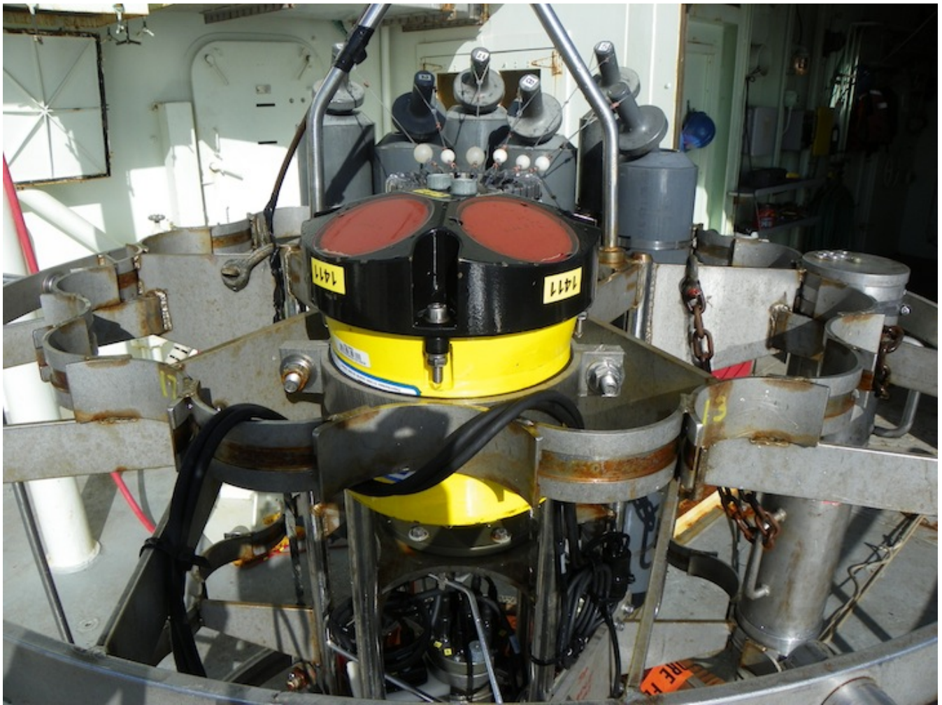
This is a close-up of the LADCP on the top of the CTD frame. You can see the open Niskin bottles behind it. © Pat Keoughan
