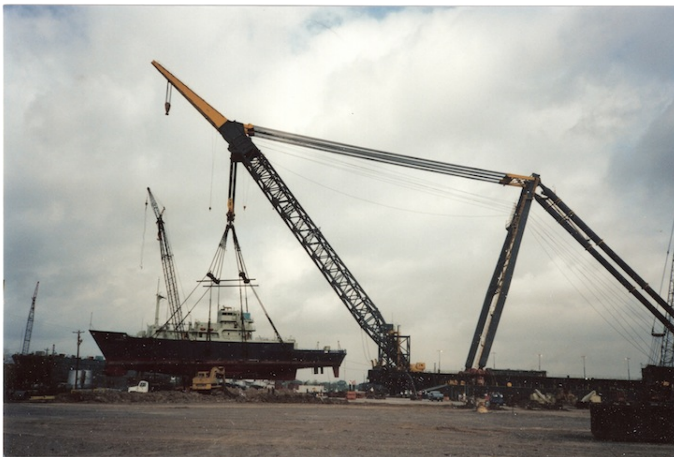
The smaller Knorr is eased onto blocks by a complicated crane. You can see where the crane's wires are attached to the lift points on the Knorr. (Credit: Wayne Sylvia)
