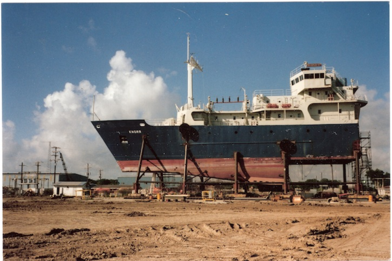
QS8_05c.JPG The bow half of the Knorr, looking very odd, sits on blocks at the McDermott Shipyard in Amelia, Louisiana, US. (Credit: Wayne Sylvia)
