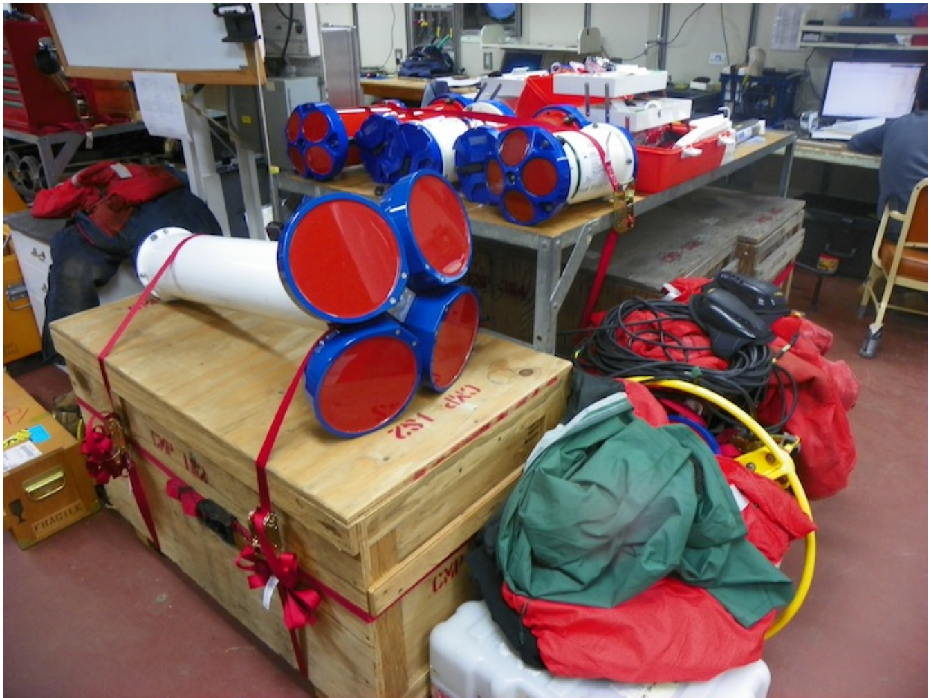
Small and large ADCPs are secured in the Knorr's main lab until they are used on moorings during the cruise. They will measure the velocity (speed and direction) of the currents passing the mooring for the next year. © Pat Keoughan
