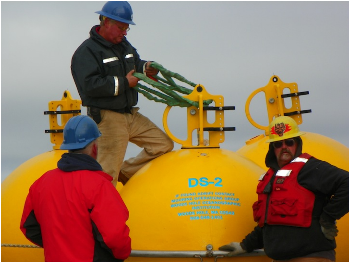
Mooring technician John Kemp, with the help of mooring team member Jim Ryder and bosun Kyle, readies one of the floats to be lifted by crane and moved to the edge of the transom. From there it will be lowered into the ocean. © Pat Keoughan
