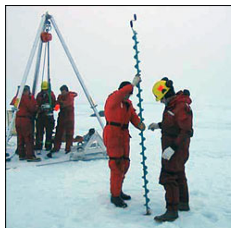
Drilling 11" diameter hole for ITP deployment on the left and 4" diameter hole for IMB on the right.
