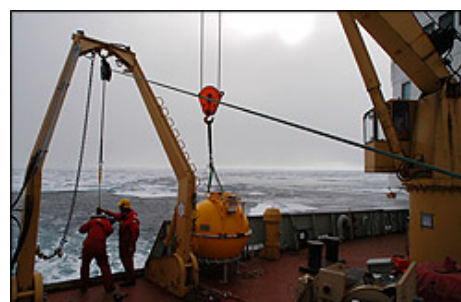
Rick Krishfield and Doug Sieberg attach the top bumper for the moored profiler.
