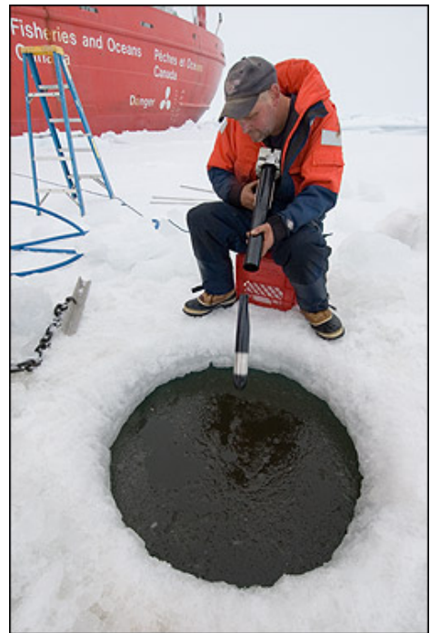
John Kemp launches an XCTD through the melted hole. The falling probe is visible just above the water's surface.
