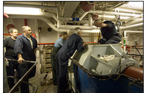
An expectant crowd gathers around the starboard shaft as Senior Engineer Stephen Hewens (far right) uses a magnet to retrieve metal pieces from the oil-filled space.
