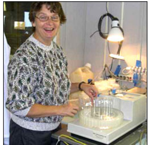
Linda White operating the auto-analyzer for measuring nutrients.
