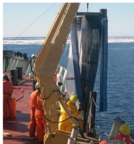
The bongo net being deployed by Amanda Byrd using the forward A-frame.
