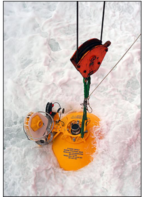
The ship's bubblers froth up the water as the top sphere is about to be released.
