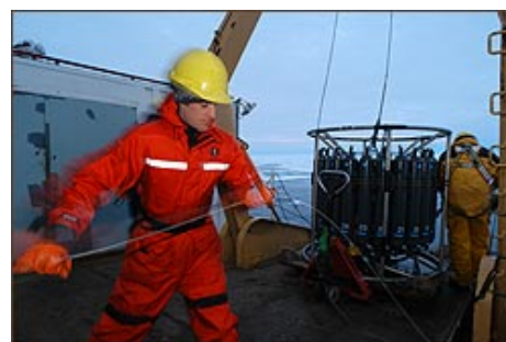
Cleaning up after the CTD cast; Ryan North (left) takes up the CTD conducting wire while Hugh Maclean (right) reattaches the lifelines.
