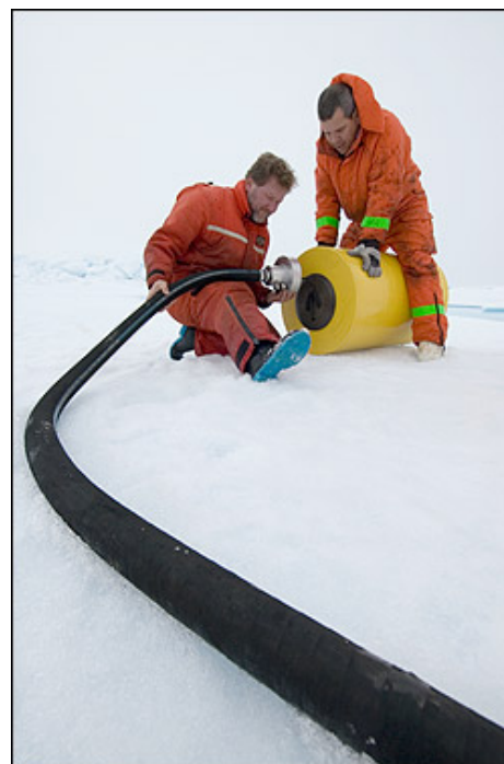
Rick Krishfield (left) and Peter King finish assembling the ITP top float.
