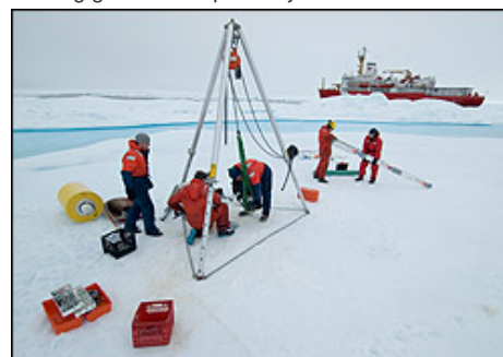
Assembly of the ice-tethered profiler (foreground) and the ice mass balance buoy (background).
