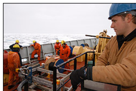
Kris Newhall drives the Lebus winch, which slowly lowers the mooring during the deployment.
