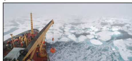
Mooring A's top sphere is lowered into the water using the crane. Notice the size of the open water area created by the bubbler system.
