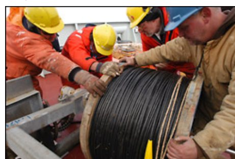
Teamwork is critical for large mooring deployments like this one. Here the team loads a 1500 pound spool of wire.
