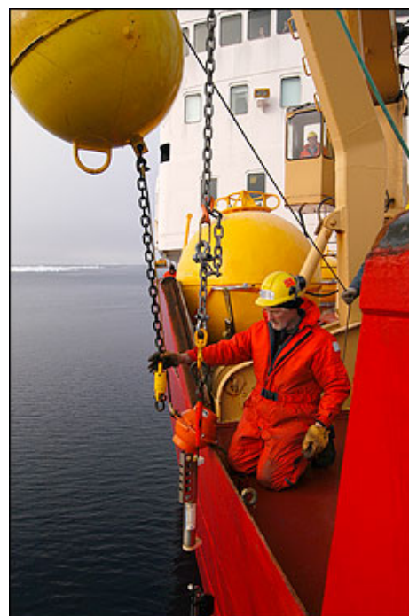
IOS Chief Technician Doug Sieberg inspects the CABOS mooring as it is reeled in.
