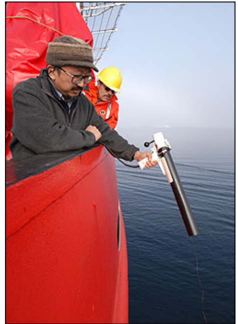
Masuo Hosono from the Japan Marine Science and Technology Center (JAMSTEC) launches an expendable CTD, or XCTD. XCTDs will be used to augment our regular CTD sampling.
