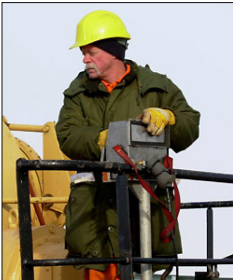
Seaman Bill May carefully watches the wire on the Lebus winch while operating the controls during a mooring operation.
