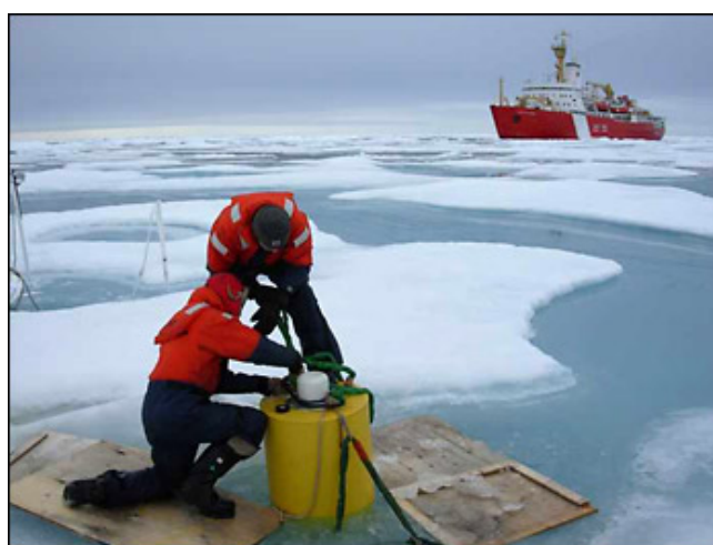
Will Ostrom and Kris Newhall attach slings to the ITP top float so that the ship's crane could be used to take hold of the system. Photo by Rick Krishfield, WHOI.
