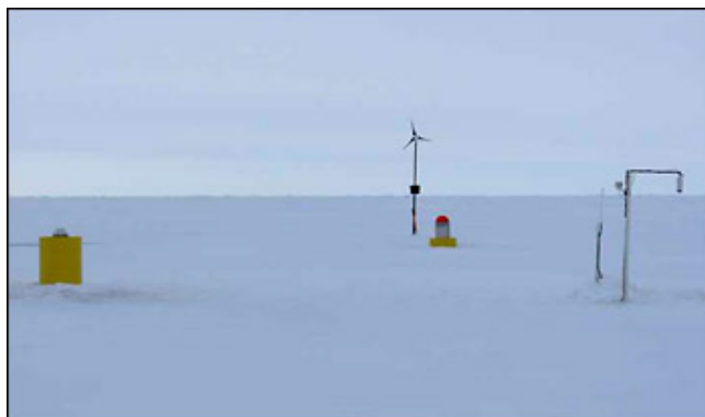
The Ice-Based Observatory after installation. The ITP buoy is on the left, the AOFB buoy is in the center (with wind generator for additional power), and the IMB is on the right. Photo by Rick Krishfield, WHOI.
