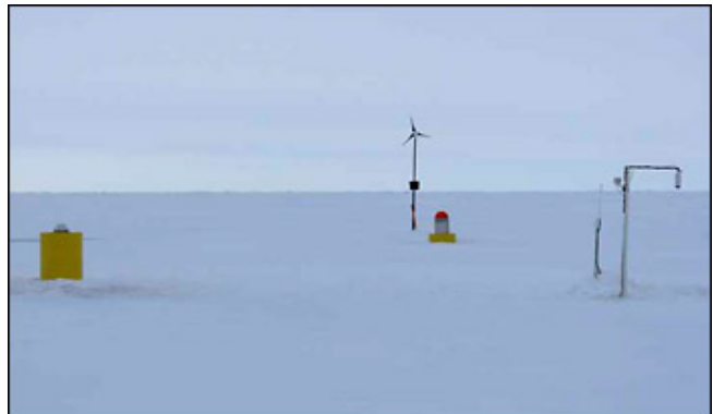
The Ice-Based Observatory after installation. The ITP buoy is on the left, the AOFB buoy is in the center (with wind generator for additional power), and the IMB is on the right. Photo by Rick Krishfield, WHOI.
