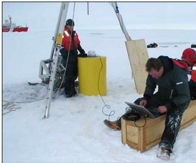
Kris Newhall stands by the ITP buoy while Rick Krishfield connects to the instrument to verify proper communications between the surface package and profiler. Photo by Gary Morgan.
