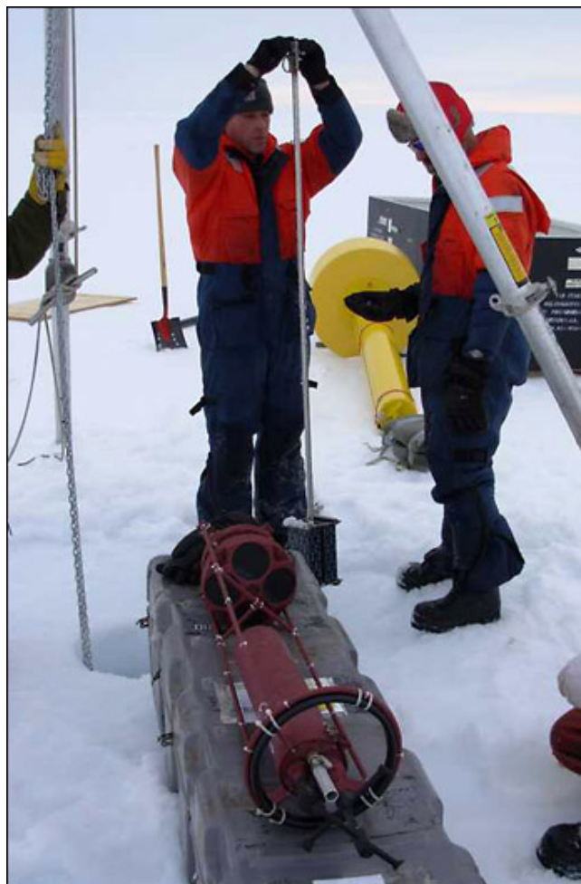
Kris Newhall and Will Ostrom rig the bottom segment of the AOFB for deployment. The red package in front of them includes the temperature, conductivity, and velocity sensing elements. The yellow package behind them is the buoy top which includes the GPS locator and Iridium communications systems. Photo by Rick Krishfield, WHOI.
