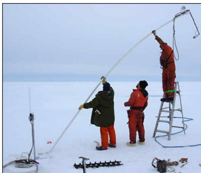
Bill May, Mike Dempsey, and Gary Morgan hoist the snow sensor for the IMB into place. On the left, you can see the buoy package with transmission antenna. Photo by Rick Krishfield, WHOI.
