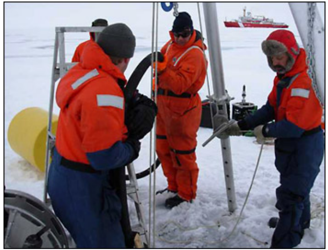
Kris Newhall and Brian MacKenzie guide the reinforced cable, while Will Ostrom slips the ITP buoy over the ice hole to cap the mooring. Photo by Rick Krishfield, WHOI.
