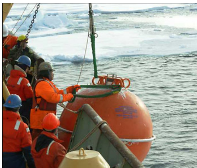
Rico Amamio rigs the top sphere of the mooring for deployment. Once the top sphere is released, the mooring will settle into position, tethered to the ocean bottom for another year. Photo by Rick Krishfield, WHOI.
