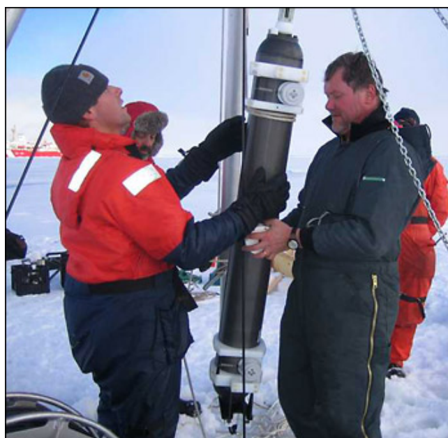
Kris Newhall and Rick Krishfield attach the ITP profiler to the wire. Photo by Chris Swannell.
