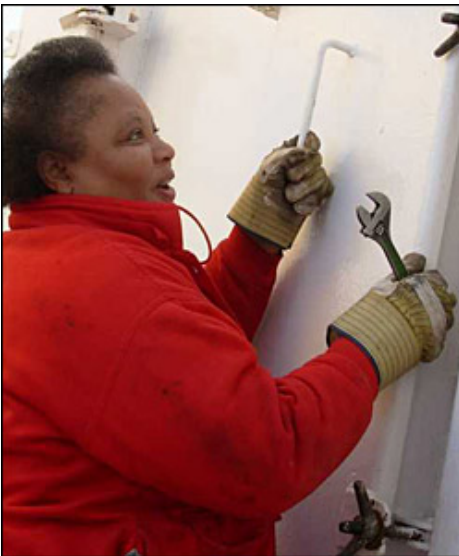
Engine Room Mechanic Raine Jones secures one of the foredeck vents for the blowers.
